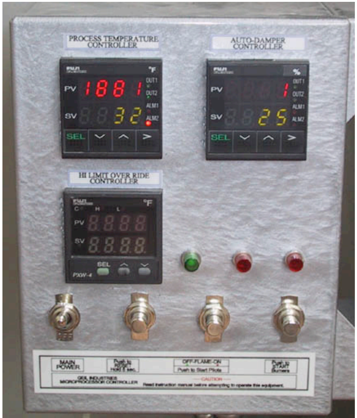
Figure 1: The Control Panel for the Automated Kiln
